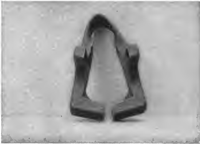
FIG. 3.—C-46-O Krupp steel chassis frame cross member. Flattened down under the hammer with no sign of cracking.
